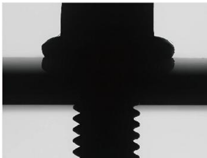
尺寸、无牙、斜牙、烂牙 Dimension, non-threaded, skewed thread, damaged thread
