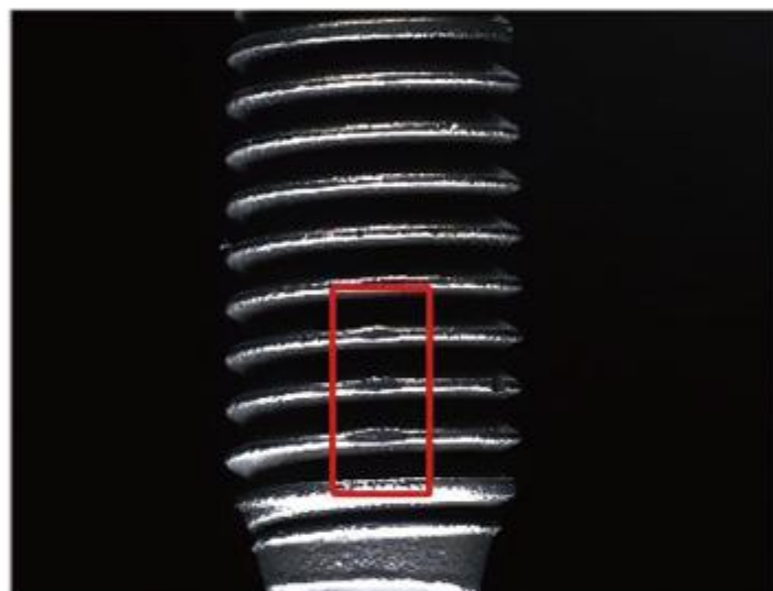
牙伤 Thread damage
