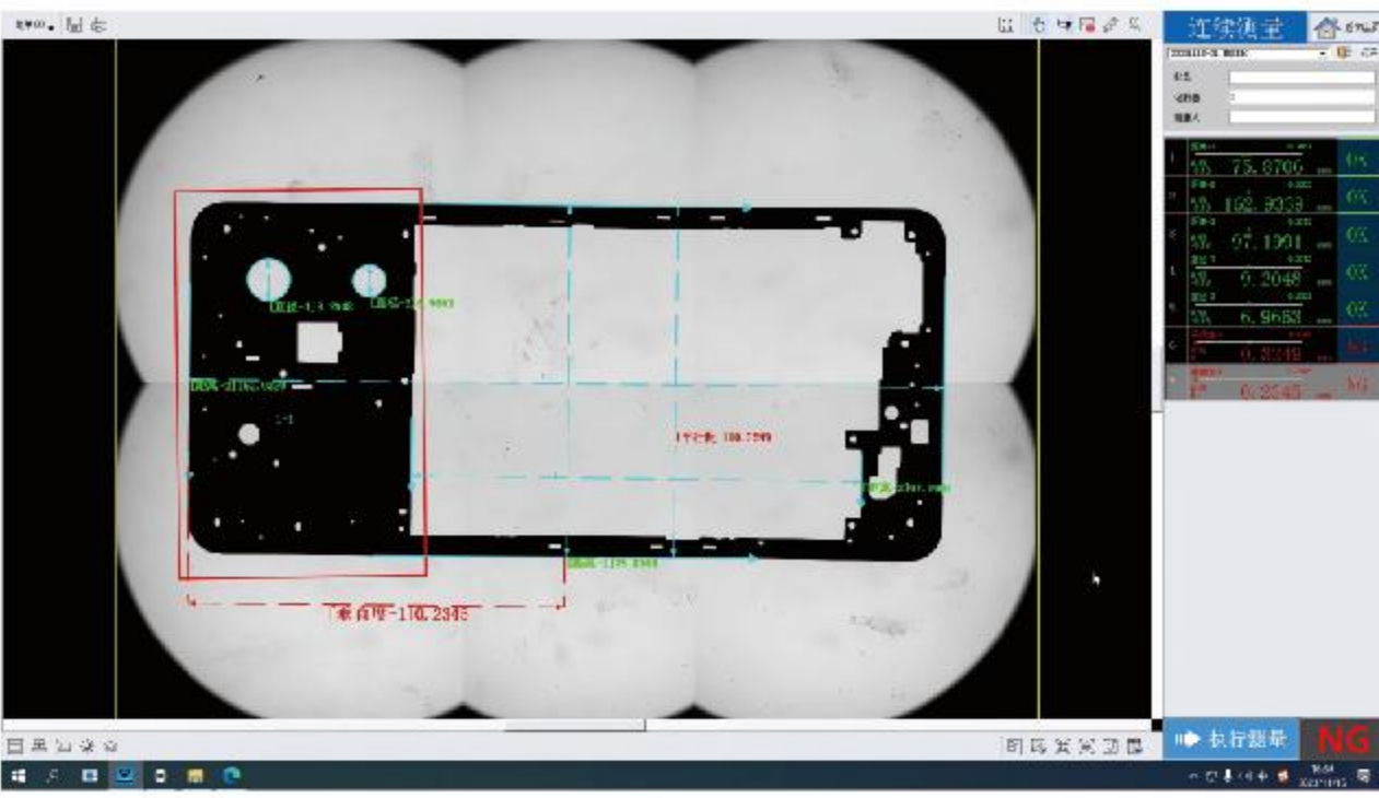
广视野模式拼接成像-手机中框 Wide-FOV Mode Image Stitching-Phone Midframes
