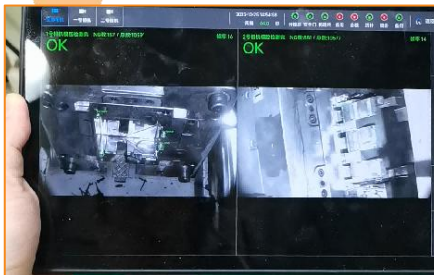
New energy vehicles - Detection of abnormalities in metal fittings embedded in the battery box
