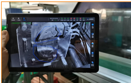
Automotive parts - detection of abnormalities in the removal of parts from molds by mechanical hand
