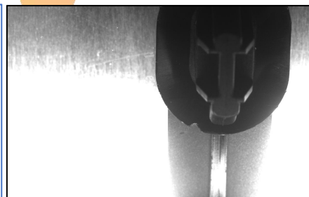
Car snap - edge shortage of material
