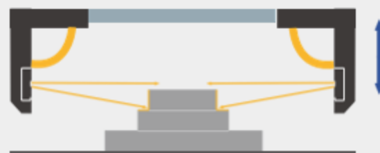
缝隙环状照明照射时截面面积
